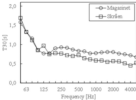
Fig. 2.  $T_{30}$  of the two venues, *Magasinet* and *Skrâen*, including audience calculated with absorption coefficients from [1].
