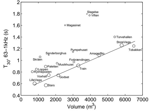
Figure 4: Mean measured  $T_{30}$  for the 63 Hz to 1 kHz octave bands vs. hall volume for the twenty halls in the study (empty halls). A larger marker indicates a better ‘General Rating.’ The line shows a recommended guide for the reverberation time for a given hall volume.
