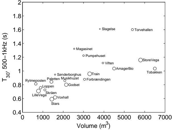
Figure 3: Mean measured  $T_{30}$  for the 500 Hz and 1 kHz octave bands vs. hall volume for the twenty halls in the study (empty halls). The size of the marker indicates the general rating of the hall with better ratings having larger markers.
