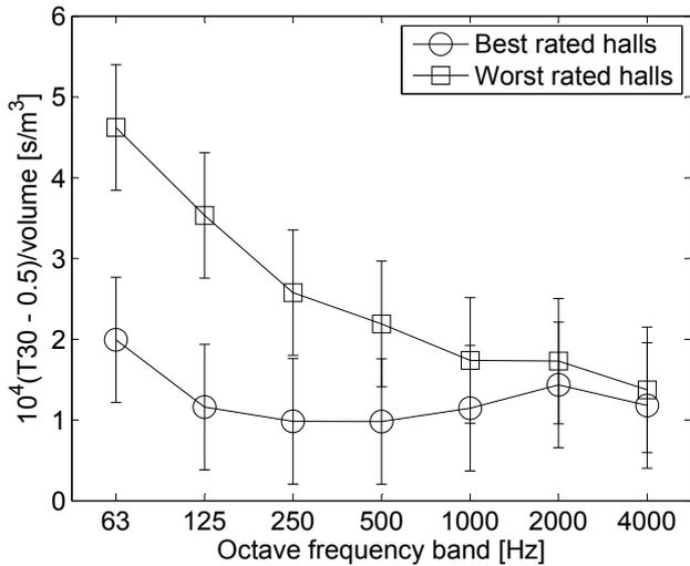
Figure 5: Linear transform of  $T_{30}$  by volume as a function of frequency band, grouped by best- and worst-rated halls. Shown are the estimates of the means of  $(T_{30}-0.5s)/Volume$  and 95% confidence intervals for the two groups.
