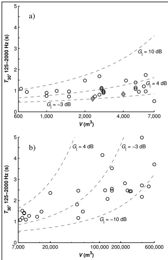
Figure 2: Calculated reverberation time ( $T_{30}$ ) as a function of volume ( $V$ ) of a) small and b) large venues.
