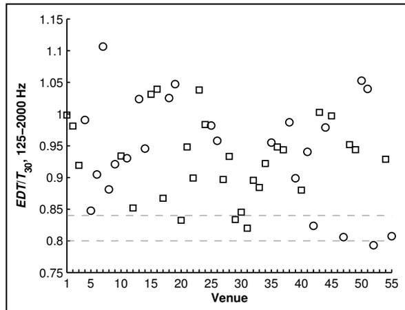
Figure 4: Calculated  $EDT/T_{30}$  for the 55 venues.
