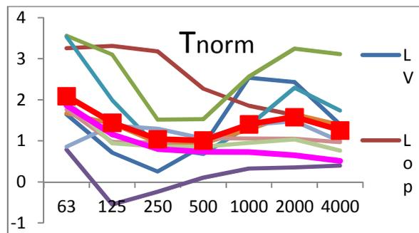
Figure 4: Measured  $T_{30}$  for ten best halls [1] normalized with respect to their volume
