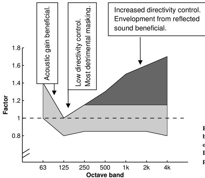
Fig. 5: Approximate factors of  $T_{30}$  in the octave bands 63 Hz to 4 kHz relative to average value of  $T_{30}$  within 125 to 2 kHz as proposed in fig.3. Light grey area: tolerances as debated in this paper. Dark grey area: possible tolerances.
