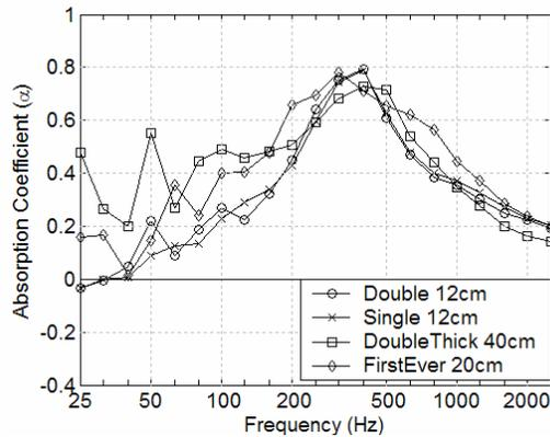
Figure 2 Absorption coefficients of 4 air mattresses
