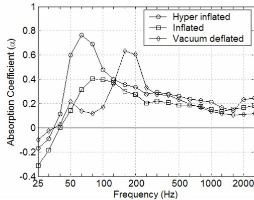
Figure 3 Absorption coefficients of 2mm PVC on testbox
